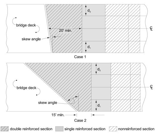
Figure 1: Case 1 and Case 2 bridge approach section layouts.
