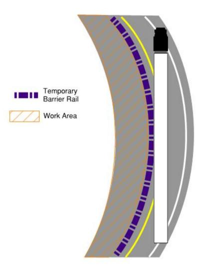
Obstructions such as temporary barrier rail or channelizers can pose a unique challenge when placed on the inside of a curve. While some long loads may fit the available width at any point along the curve, they may be too long and become stuck as shown in the example above. In these cases, a length restriction should also be calculated and reported to the 511 system.
