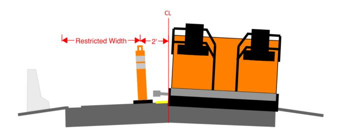
Iowa DOT specifications allow the contractor to place channelizers up to two feet beyond the centerline. The restricted width should account for this extra space to protect the equipment and the people working just on the other side of the channelizers.
